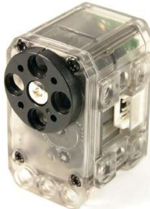
Figura 3.14 – Servo-motor dynamixel XL320
