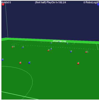
Fig. 1. The current version of the 3D simulation using spheres as agent models. Every agent has an omni-vision camera which delivers noisy data about the environment, a kick-effector to shoot the ball, and an actuator simulating omni-drive to move on the field.
