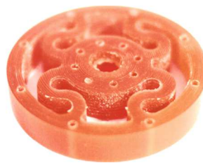
Fig. 2. Polyurethane spring proposed in our system (Color figure online).
