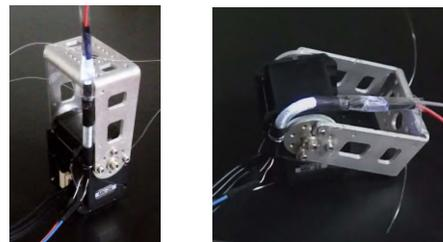
(a) Actuator at 180°. Sensor extended. (b) Actuator at 60°. Sensor flexed.
