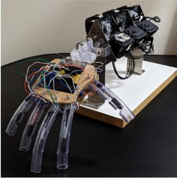
Fig. 7: Fully constructed hand with sensors attached.
