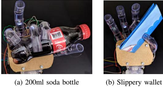
Fig. 11: Gripping of a heavy and a slippery object.
