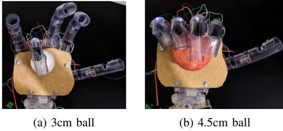
Fig. 10: Gripping balls of different sizes.
