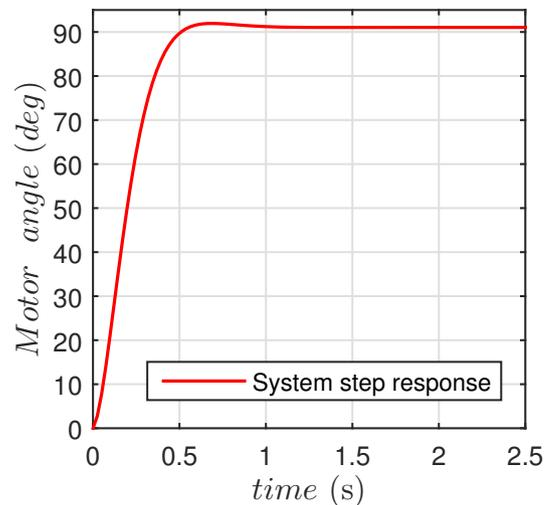
Fig. 13. Step response for simulated dynamixel motor.
