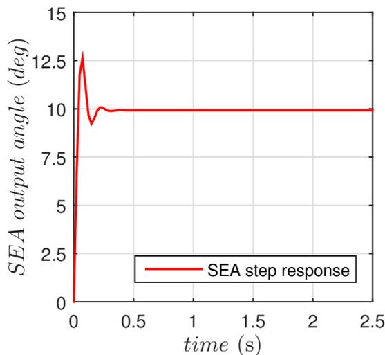
Fig. 11. Step response for the simulated SEA system.
