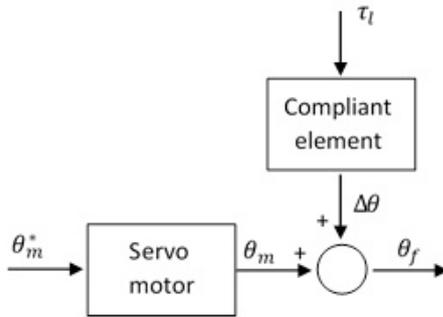
Fig. 6. Typical impedance control loop.
