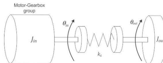
Fig. 1. Series Elastic Actuator Topology (Laffranchi et al., 2011)
