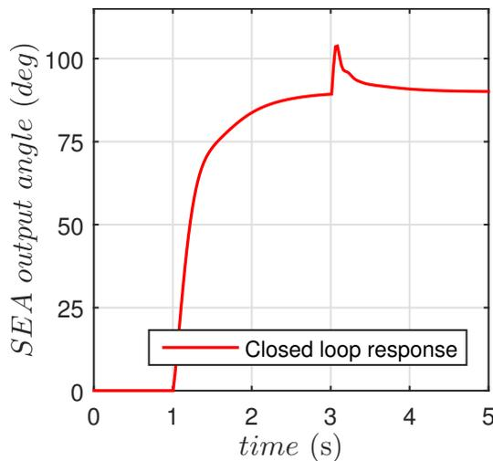
Fig. 16. Compensated system response showing how the closed loop SEA system is now capable of rejecting the same external disturbance.
