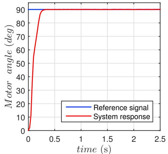
Fig. 12. Step response for real dynamixel motor.
