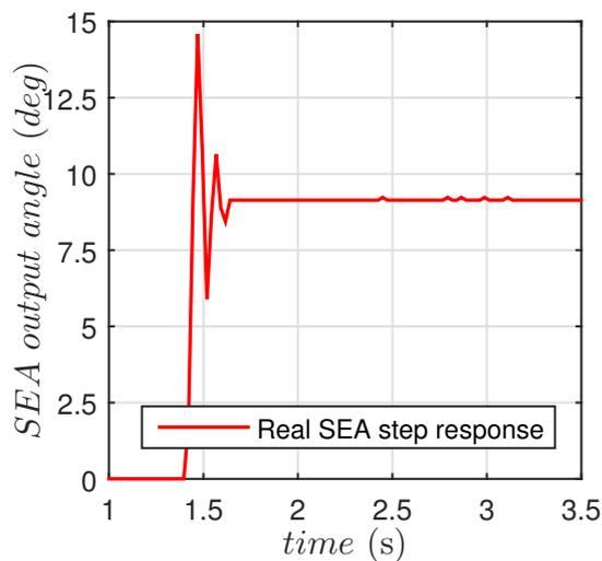
Fig. 10. Step response for the real SEA system.
