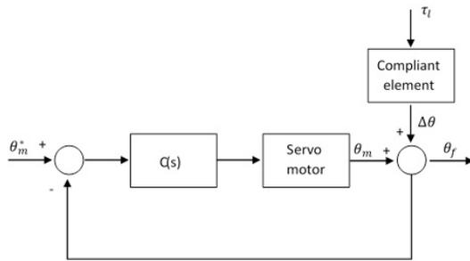
Fig. 8. Typical impedance control loop.
