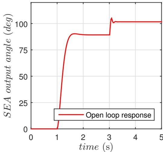
Fig. 14. The uncompensated system shows an steady state error when load is applied.
