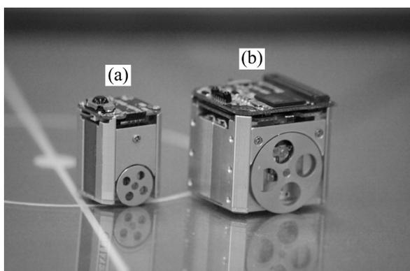
Fig. 6 Close-up picture of the two micro-robot versions, (a) the version used in our experiments so far, and (b) the newer version with more powerful embedded microcontroller and longer battery life at the expense of an increased body size. The faster processor allows installation of embodied devices such as speakers and microphones for production and detection of chirping.
