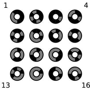
Fig. 2 Figure showing the patterns of circular bar code that are used for localization.
