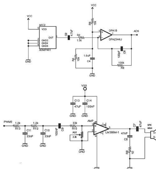
Fig. 7 Extensions being designed for the new robot. On top the circuit of the microphone and on bottom the circuit of the speaker.
