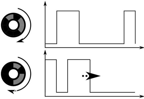
Fig. 1 After the center of each marker is located a 16 bit binary pattern is sampled from a disc with pre-define radius. Based on the pattern and its offset the agent's id and orientation are respectively obtained.
