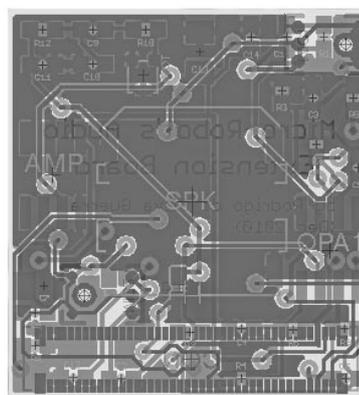
Fig. 8 Design of the micro audio extension board. On the top right one microphone, on the bottom left another. Speaker in the center.
