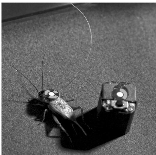
Fig. 5 Picture of cricket interacting with micro-robot, while EMG signal is captured live through a thin cooper wire attached to its mandible muscles.
