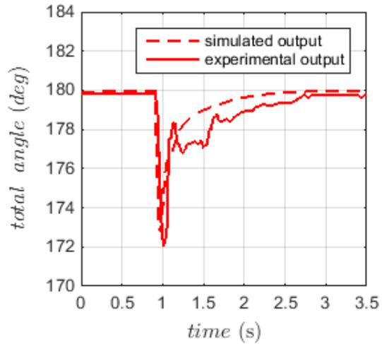
**Figure 6: Closed loop response releasing weight at a specific time.**
