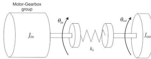
**Figure 1 - Series Elastic Actuator Topology.**
