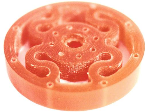
**Fig. 7** Manufactured polyurethane-based torsional spring
