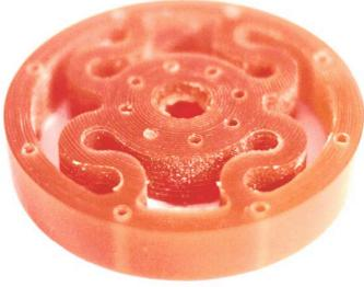
Fig. 4: Manufactured polyurethane-based torsional spring.
