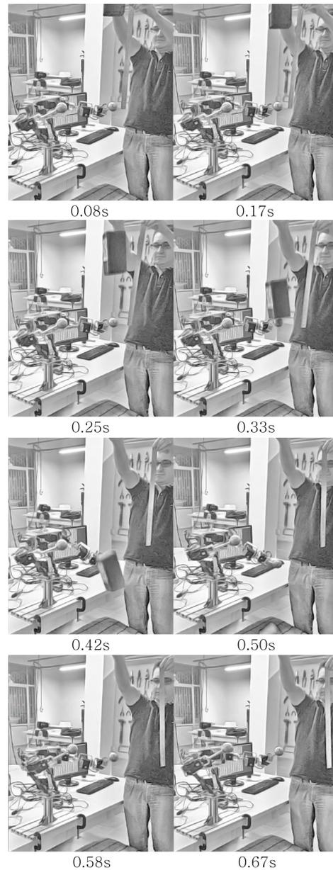
Fig. 8: A 2.57kg brick is dropped from a height of 50cm over Dimitri's left arm, causing no damage. The robot recovers the original posture less than a second later.
